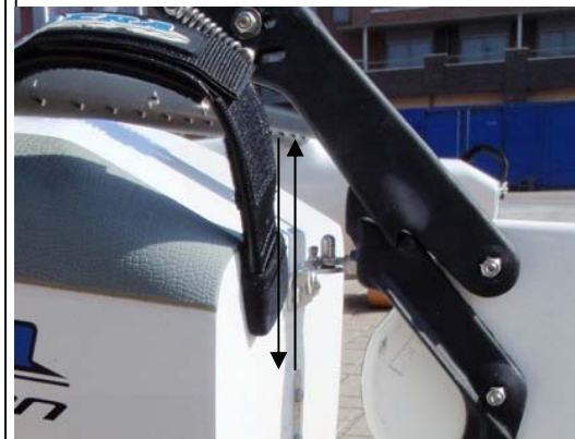
Step 6 Locking the rudders part 1
