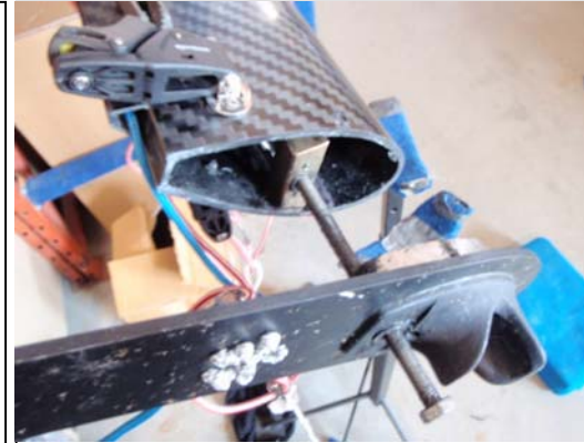
Step 5 Grease the bolt! Only get the thread started!
