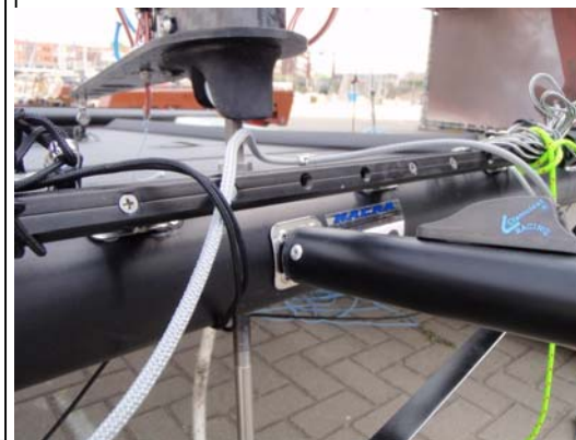
Step 1 Jib sheet on top of spinnaker pole!
