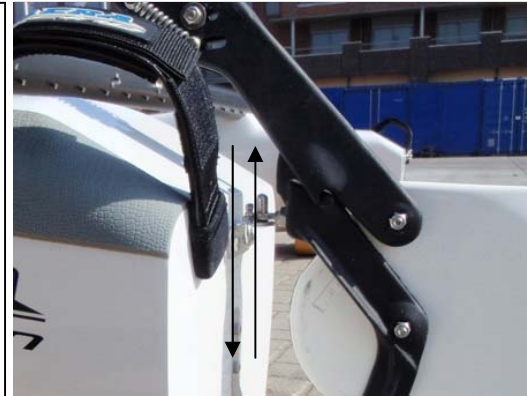
Step 6 Locking the rudders part 2 The rudder is now locked.
