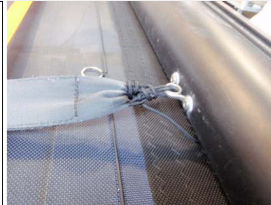
Fixing the foot straps Step 1
