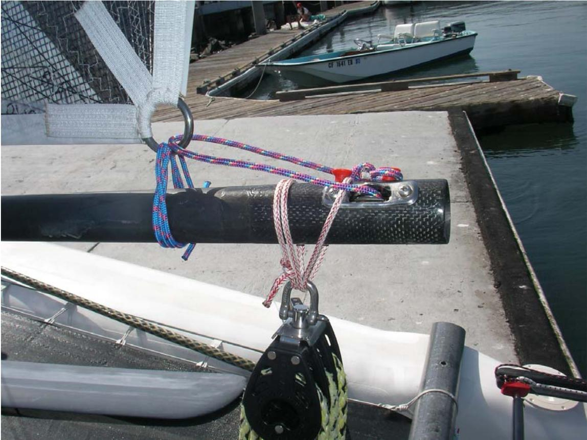
Mast raising and lowering – To raise the mast, attach the mast raising hinge plate on the mast ball to the mast base fitting on the main beam with a clevis pin. Make sure there is a ring ding or other device to keep the clevis pin from accidentally falling out. The mast head should be pointed forward. You will want to place the masthead on a sawhorse or other suitable support.
